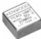
SO-2 Temperature- compensated Crystal Oscillator (TCXO)
